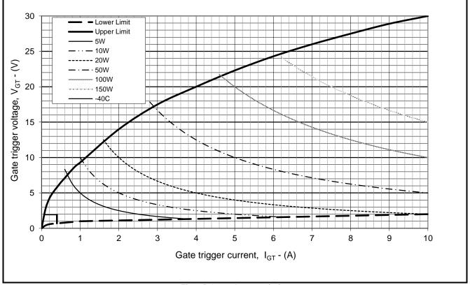
Fig. 15 Gate characteristics
