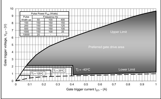
Fig14 Gate Characteristics
